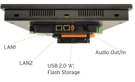
you can have one port dedicated for machine communications over Ethernet, such as I/O, third party devices, PLC networks, any other factory-level communications, and now a second Ethernet port is separate and isolated to interface with the wider factory information systems, such as SCADA, ERP, MRP, or other factory networks for sending email or transferring files.
