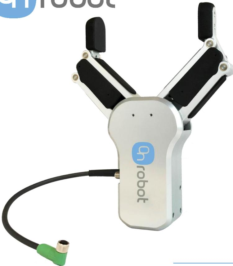
The RG6 gripper is a flexible electric gripper specially designed for robots from Universal Robots. The long stroke allows the gripper to handle a variety of object sizes. Adjusting the gripping force allows the gripper to handle both delicate and heavy object. The standard fingers can be used with many different objects, it is also possible to fit custom fingers.
