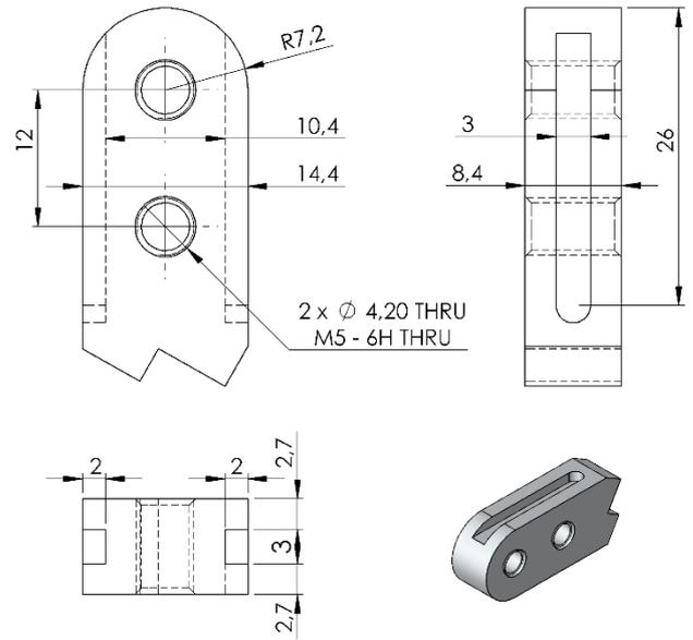
Dimensions of the gripper aluminum finger tips.
