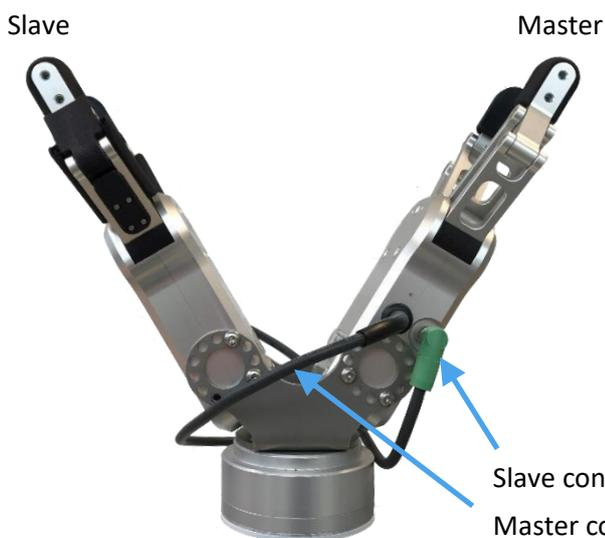
When one gripper is connected to another via the gripper output connector, the first gripper in the chain (from the robot) becomes master and the second slave.
