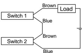
When two switches are connected in series, a load may malfunction because the load voltage will decline when in the ON state. The indicator lights will light up if both of the switches are in the ON state.
