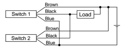
The indicator lights will light up when both switches are turned ON.
