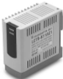
The regenerative absorption unit absorbs the energy (regenerative energy) that is generated by the motor when it decelerates. It is used to prevent drive power abnormality in the controller.
