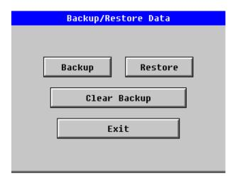
Backup = Copies Battery Backed RAM contents on to the onboard FLASH memory of the OCS.
