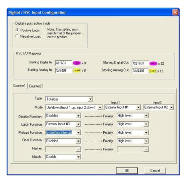
Figure 15.2 – Digital Input / HSC Configuration Dialog
