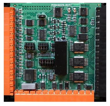
Figure 10.3 - XL4 I/O Cover Removed (sample I/O board)
