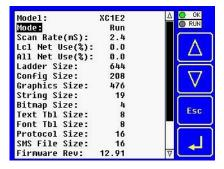
The View Status Sub-Menu displays up to 19 System Settings. Only the **Mode** System Setting is editable.
