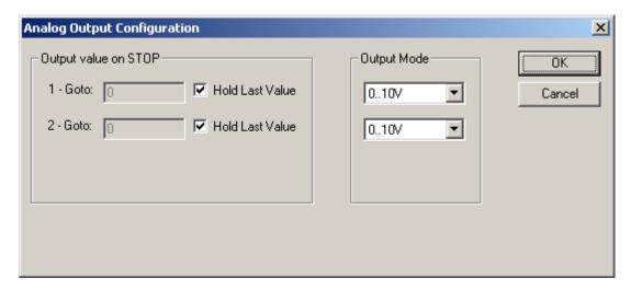
Figure 15.5 - Analog Output Configuration Dialog
