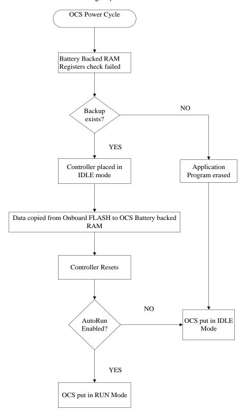
Figure 16.6 - Flow Chart for Automatic Restore
