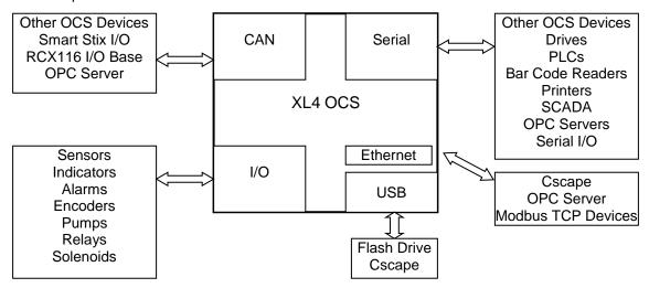
Figure 2.3 – Visual Overview of Types of Devices that can be connected to XL4 OCS
