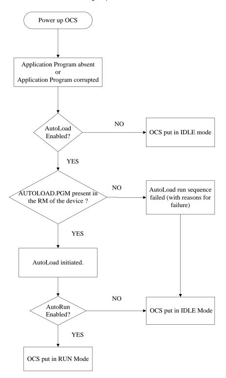
Figure 16.8 - Flow Chart for AutoLoad
