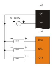
Figure 10.5 - Typical Output Wiring
