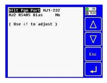
The Set Serial Ports Sub-Menu displays three System Settings, all of which are editable, and one optional item. For the **Dflt Pgm Port** System setting, only MJ1-232 can be selected, unless a Modem (XMC) COM module is installed.
