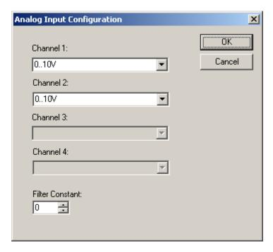
Figure 15.4 – Analog Input Configuration Dialog
