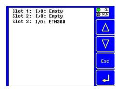
The View I/O Slots Sub-Menu displays three System Settings, all of which are not editable.
