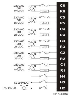
Figure 10.6 - Relay Fusing
