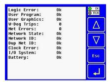
The View Diags Sub-Menu displays up to 11 System Diagnostics, none of which are editable.
