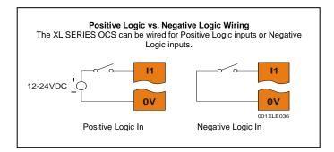
Figure 10.7 – Positive and Negative Inputs
