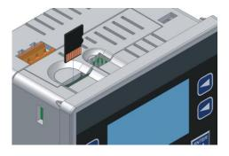
Figure 9.2 – Installing Removable Memory Card
