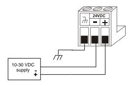
Figure 4.2 – Power Connector (Primary Power Port)
