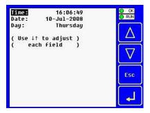
The Set Time/Date Sub-Menu displays three System Settings. **Time** and **Date** are editable, and **Day** is automatically calculated from the **Date** setting. Note that **Time** and **Date** are split into three editable fields each. Use  $\leftarrow$  or  $\rightarrow$  to select a field and then use  $\downarrow$  or  $\uparrow$  to edit the field.
