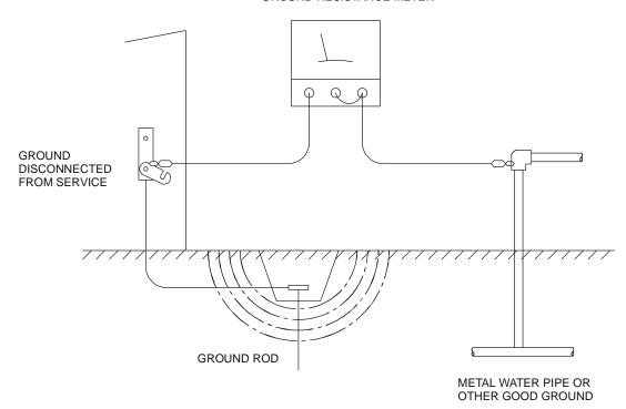
Figure 4.1 - Two-Point Ground Connection Test
