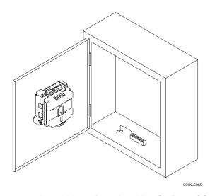
Figure 3.1 - Panel Mounting of an XL4 Series OCS
