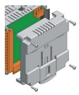
Figure 10.1 – Removing the I/O Cover
