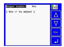
The Set Beeper Sub-Menu displays one System Setting, which is editable
