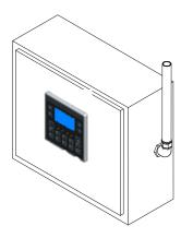
**NOTE:** For panel or DIN rail mounting: The orientation shown above provides for <u>optimum readability</u> of the screen and <u>ease of use</u> of the keypad.
