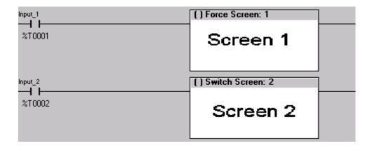
Figure 13.4 - Force and Switch Coils in Ladder Programming
