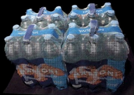
3D scan with color texture showing 4 six-packs of plastic bottles in transparent foil
