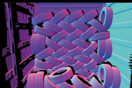
3D scan with normals showing a stack of black tires scanned from 4 m / 13,1 ft distance
