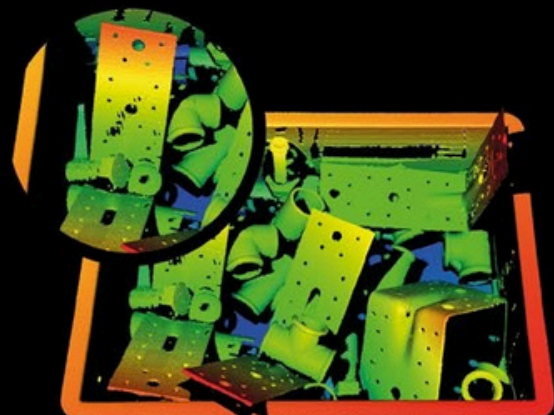
Point cloud colored with depth map showing unstructured mixed bin filled with reflective metallic parts
