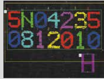
Optical character reading Dot matrix printing can also be read with OCR.
