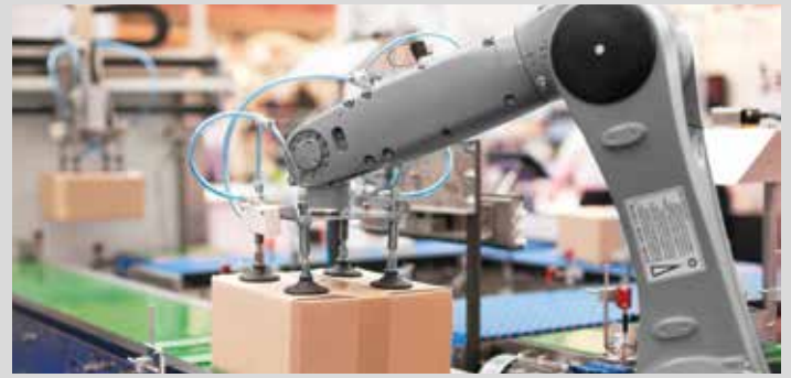
Determining the position of a package so that it can be gripped by a robotic arm
