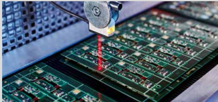
Detection of double layers on printed-circuit boards, or checking the height and presence of components
