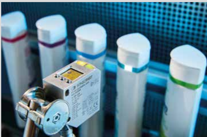
Color detection of packaging elements
