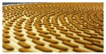
Maintaining the buffer zone around each bar is important because the machine vision systems cannot recognize one or more bars if they are touching each other. Overlapping or occluded bars lead to missed picks and wasted product. Unfortunately, when a robotic arm fails to cleanly pick a bar or drops it during transport to the lug conveyor, the bar often ends up touching another bar, doubling the amount of waste.
