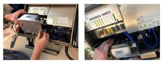
3. Carefully insert the SRCU-Mini UR+ so as to not damage pneumatic fittings or any electrical connectors. Orientation for insertion is referenced in above photos.
