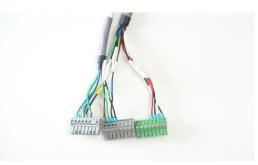
1. Remove Universal Robot Controller Terminals "Analog", "Digital Inputs" and "Digital Outputs", that correspond with below wiring diagram, from the Universal Robot Controller.
