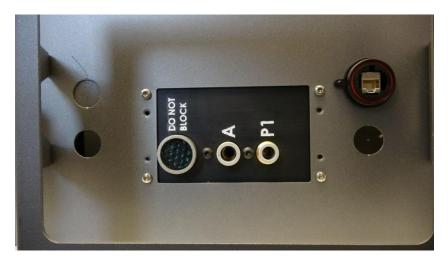
1. Cut and connect ~50mm of the provided 10mm and 12mm tubing to the exposed SRCU-Mini UR+ fittings. 10mm tubing connects to "**P1**" and 12mm tubing connects to "**A**." Ensure tubing is secure in ports.
