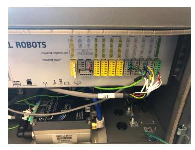
3. Reconnect terminal strips to appropriate locations on Universal Robot Controller.
