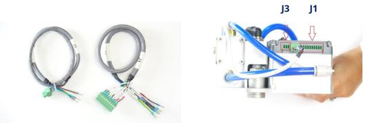
1. Install cable harnesses into SRCU-Mini UR+ controller. "J3" is the power cable, and "J1" is IO. See Section 1E: Product Overview for additional depiction of the SRCU-Mini UR+.
