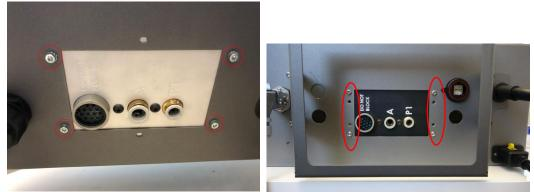
4. Re-use the UR Controller Cabinet access panel screws to mount the SRCU-Mini UR+ to the cabinet. Please note, depending on your Universal Robot series, your access panel may have (8) or (6) holes.
