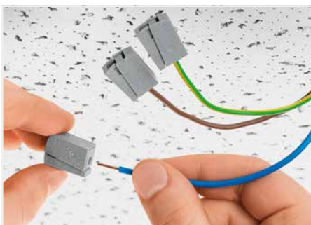
To connect: Insert stripped solid conductor into circular entry and push until it hits the backstop.
