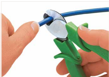
Cut the cable.
