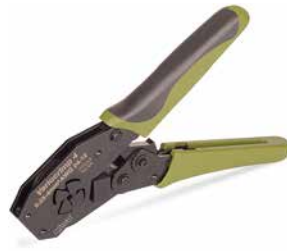
"Variocrimp 4" crimping tool; for insulated and uninsulated ferrules; crimping range: 0.25 ... 4 mm 2
