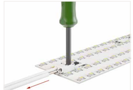
Inserting/removing fine-stranded conductors by lightly pressing on a push-button (e.g., via 206-860 Operating Tool).
