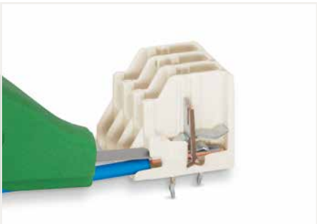
Conductor removal – PUSH WIRE®: Fully insert disconnection tool over the conductor and pull it out.
