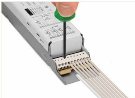
Remove the conductor by inserting a disconnection tool into the operating slot and pull it out.
