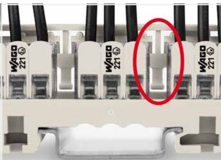
Mounting type (440 V) Using spacers between the connectors.
