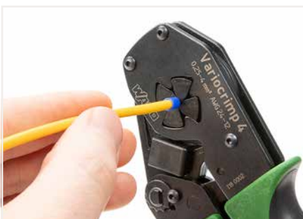
Squeeze handles until ratchet mechanism is released.
