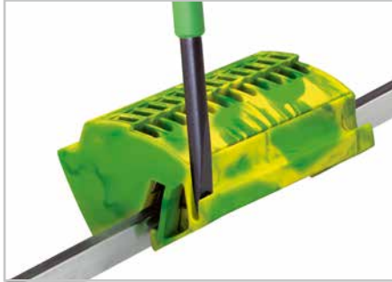
Unlock right and left positions to remove the ground busbar terminal block. Then pull up the block from the busbar.
