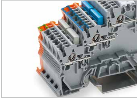
For sensor and actuator terminal blocks without ground connection to the DIN-rail, the ground connection can be performed by commoning to the terminal block with a ground foot.
