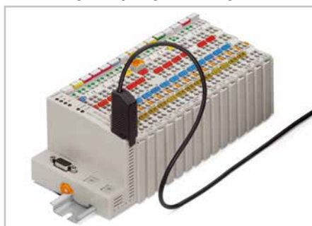
Accessing the programming interface - Programming a fieldbus controller WAGO-I/O-CHECK, WAGO-I/O-PRO CAA.
