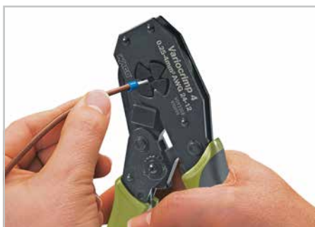
Insert ferruled conductor into crimping station. Squeeze handles until ratchet mechanism is released.
