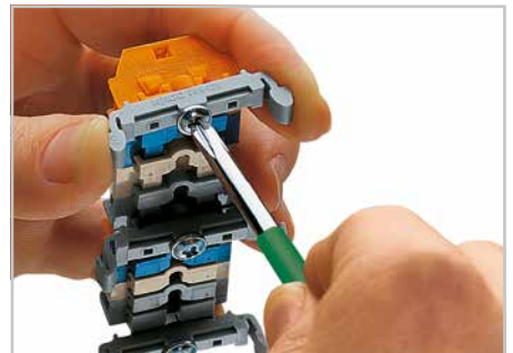
Securing a mounting foot (209-123) to the terminal strip with mounting flanges (distance between mounting feet: approx. 35 ... 40 mm).
