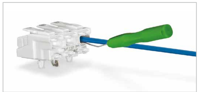
Conductor removal: Slide disconnection tool beneath the conductor and pull conductor out.
