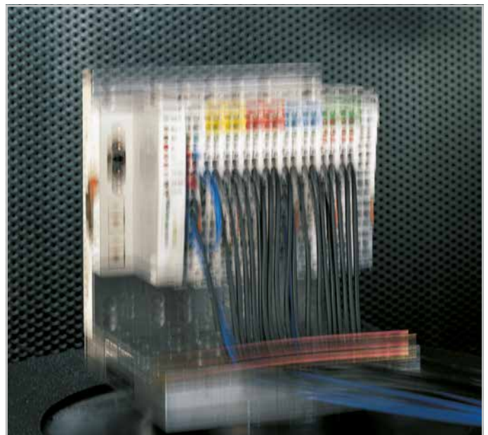
Vibration test: WAGO-I/O-SYSTEM
