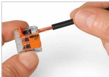
Conductor termination: Open the clamping unit using the lever and insert conductor. Then, lower the lever to close the clamp.
