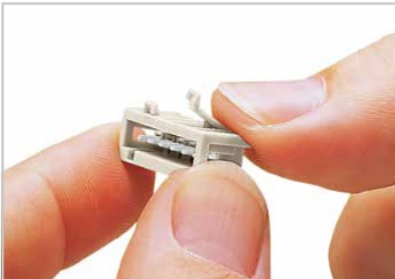
Coding a male header – fitting coding key(s).
