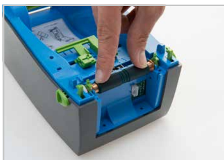
Insert and secure the suitable roller into the printer.
