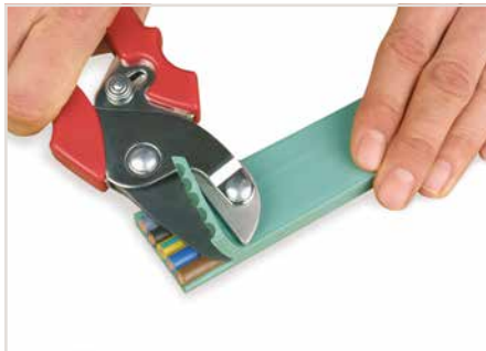
Cut off the flat cable insulation via cable cutter.
