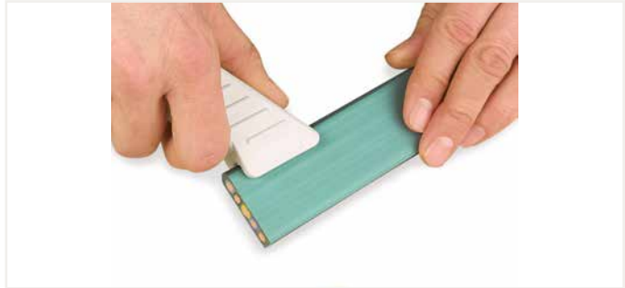
Cut both sides of the flat cable insulation using a stripping knife (observe 30 mm of cutting length).
