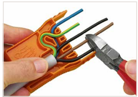
Strip outer insulation, insert cable into the wiring aid and arrange the single conductors according to the marking, starting with N. Cut conductor ends to the proper length.
