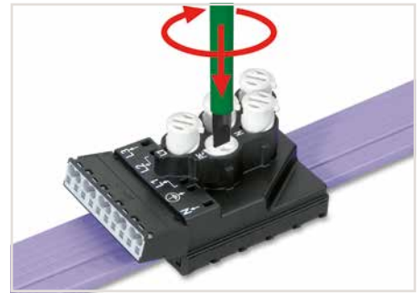
Screw down contact elements until element stops.
