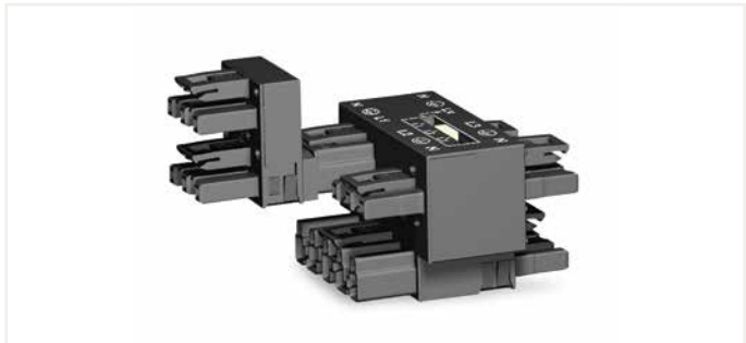
An additional h-distribution connector doubles L1. This results in the following connection options: L1/L1/L2/L2/L3 with jumper in position L2 L1/L1/L2/L3/L3 with jumper in position L3
