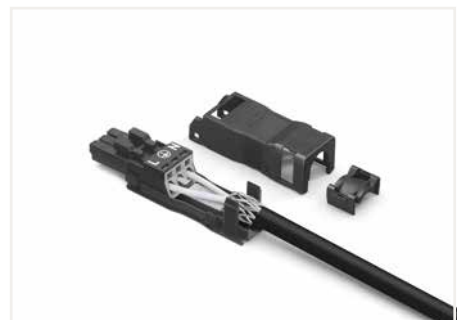
First insert the wired connector into strain relief housing, then snap clamp and cover.
