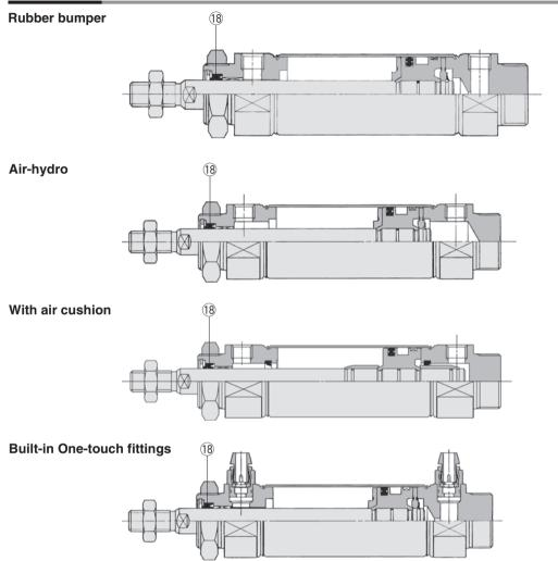
\* The numbers are the same as the "Construction" of the Best Pneumatics No.2 Series CM2.
