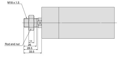
Note) Be sure to use the attached flat washers when mounting a cylinder from the rod side.
