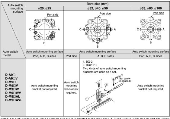
Note 1) For each cylinder series, when a compact auto switch is mounted on the three sides (A, B and C above) other than the port side of bore sizes ø32 to ø50, the auto switch mounting brackets above are required. Order them separately from cylinders. (It is the same as when mounting compact cylinders with an auto switch mounting rail, but not with ø63 to ø100 compact auto switch installation groove.) Example order
