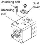
2. To use the lock mechanism again, be sure to remove the unlocking bolt.
