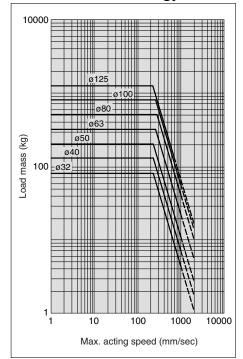
Example: Load limit at rod end when air cylinder ø63 is actuated with max. actuating speed 500 mm/s. See the intersection of lateral axis 500 mm/s and ø63 line, and extend the intersection to left. Thus, the allowable load is 80 kg.
