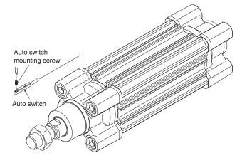
Please use a watchmaker's screwdriver with a handle diameter of 5 to 6 mm when tightening the auto switch mounting screw. A torque of 0.05 to 0.15 N ⋅ m should be used for D-M9□, M9□W, M9□AL, and 0.10 to 0.20 N ⋅ m for D-A9□. Once the screw starts to feel tight, tighten it further by approximately another 90°.
