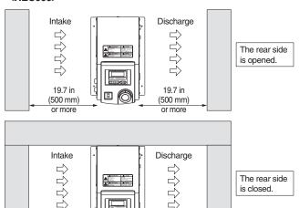
Note) The space must be 19.7 in (500 mm) or more. Be sure that the ambient temperature is within the specification range.
