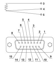
4. Alarm output connector (ALARM)
