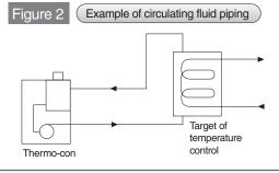
The Thermo-con is constructed as shown in Figure 1. It interposes a Peltier device (thermo-module) between the heat exchangers for the circulating fluid and facility water and controls the pulse width of supply direct current to achieve the target outlet temperature of circulating fluid precisely.
