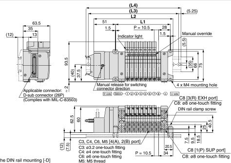
The dashed lines indicate the DIN rail mounting [-D] (with DIN rail mounting bracket).
