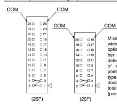
Mixed single and double wiring are available as an option. The maximum number of manifold stations is determined by the number of solenoids. Count one point for a single solenoid type and two points for a double solenoid type. The total number of solenoids (points) must not exceed 24.
