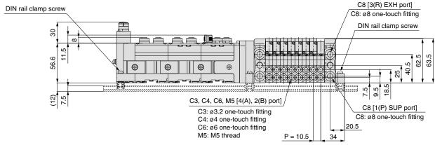
L2 = L1 - 10.5  $L3 = 10.5 \times n1 + 65.5$  $L4 = L3 + 81 + 47 \times n2$ L5 = (L1 - L4)/2 $L6 = 10.5 \times n1 + 45$
