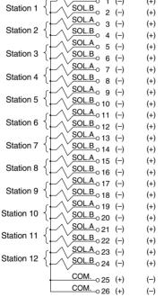
Note) When using the negative COM specification for VQC1000/2000, use valves for negative COM.
