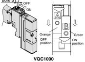
Slide the manual override button with a small flat head screwdriver or with your finger until it stops at the pilot valve side (ON side) to lock it. Slide it to the fitting side (OFF side) to release it. It can also be used as a push type using a screwdriver, etc., of Ø1.7 or less.
