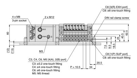
The dashed lines indicate DIN rail mounting [-D] (with DIN rail mounting bracket).
