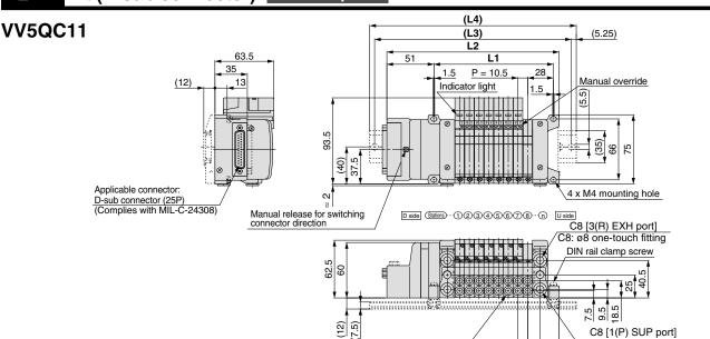
The dashed lines indicate the DIN rail mounting [-D] (with DIN rail mounting bracket).
