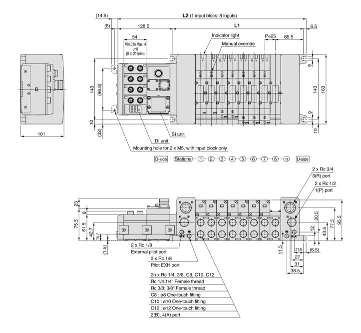
Formulas: L1 = 25n + 106, L2 = 25n + 241 (For 1 input block. For each additional input block, add 54 mm.) n: Stations (Maximum 16 stations)
