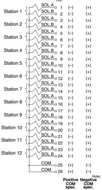
Note) When using the negative COM specification, use valves for negative COM.
