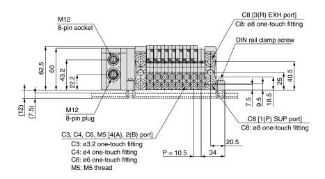
The dashed lines indicate DIN rail mounting [-D] (with DIN rail mounting bracket).
