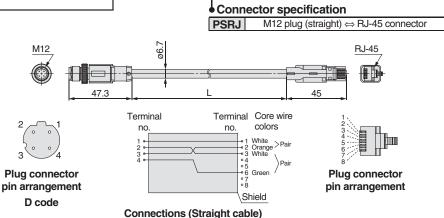
For SI units compatible with EtherCAT, PROFINET, EtherNet/IP™
