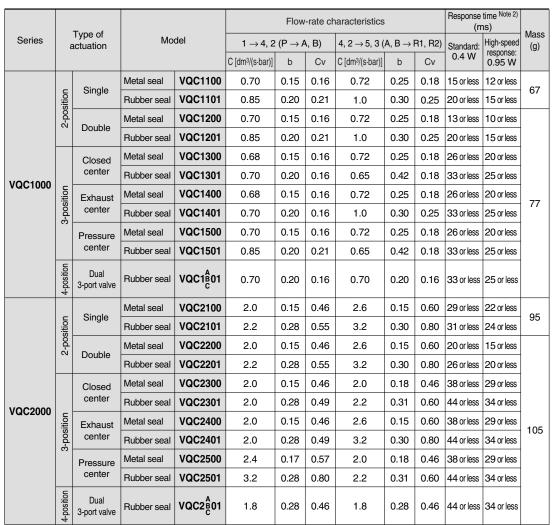
Note 1) Values represented in this column are in the following conditions: VQC1000: Cylinder port size C6 without a back pressure check valve VQC2000: Cylinder port size C8 without a back pressure check valve
