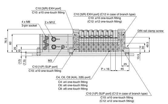
The dashed lines indicate DIN rail mounting [-D] (with DIN rail mounting bracket).
