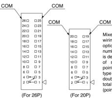
Mixed single and double wiring are available as options. The maximum number of manifold stations is determined by the number of solenoids. Count one point for a single solenoid type and two points for a double solenoid type. The total number of solenoids (points) must not exceed 24.
