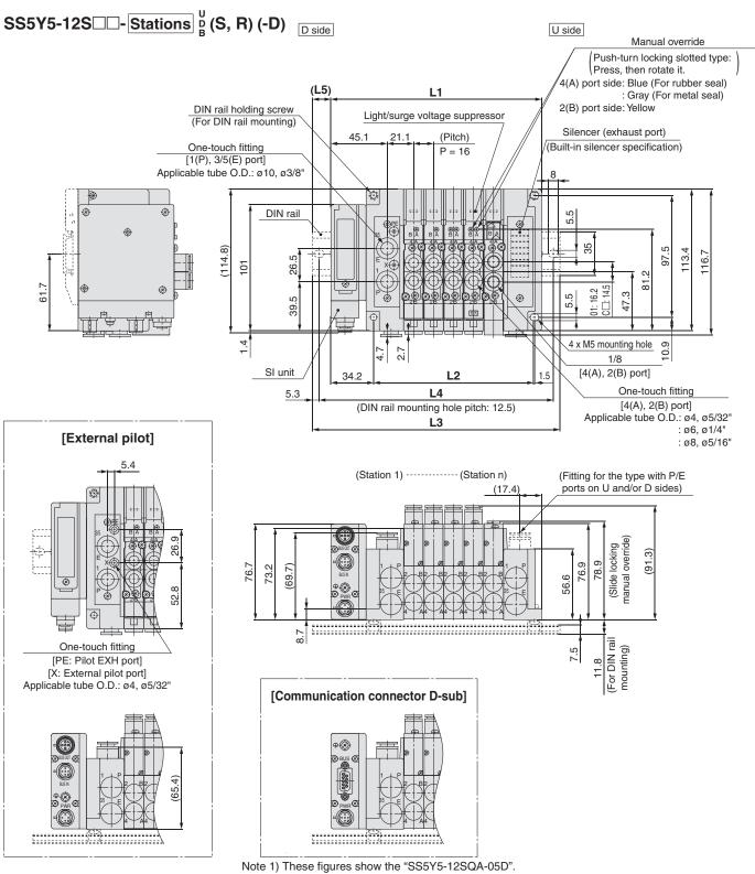
Note 2) For built-in silencer type, a silencer is mounted on the opposite side of U or D side with P or E port.
