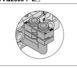
Dual flow fitting assembly VVQ2000-52A-C10
