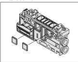
Back pressure check valve assembly [-B] VVQ2000-18A
