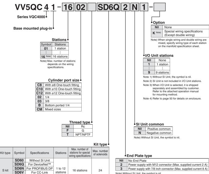
Note) Max. number of stations depends on the number of solenoids. Add the option symbol "-K" when the combination of single wiring and double wiring is specified.
