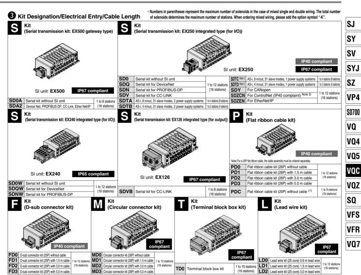
\* The maximum number of stations displayed in parentheses is applied to the special wiring specification (Option "-K").
