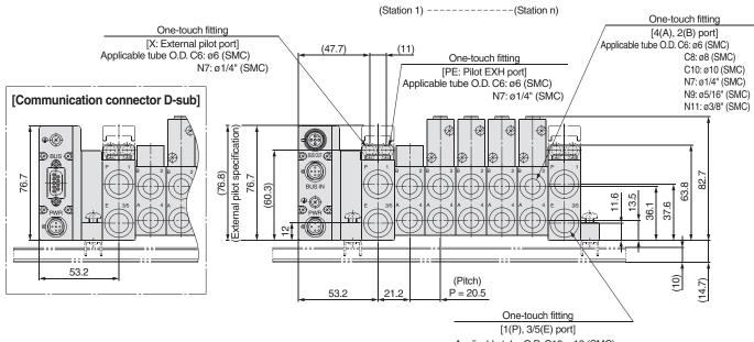
Applicable tube O.D. C12: Ø12 (SMC) N11: ø3/8" (SMC)
