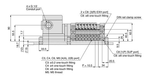
The dashed lines indicate DIN rail mounting [-D] (with DIN rail mounting bracket).
