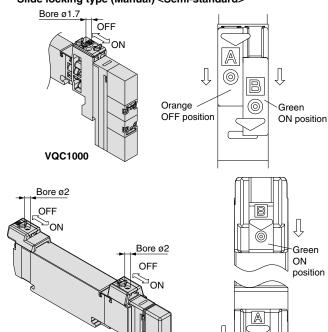
The manual override is locked by sliding it all the way to the pilot valve side (ON side) with a small flat head screwdriver or with your fingers. Slide it to the fitting side (OFF side) to release it. In addition, it can also be used as a push type by using a screwdriver, etc., of ø1.7 or less. (ø2 or less for VQC2000)
