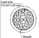
As the standard electrical wiring specification used is for 12 stations or less, double wiring (connected to SOL. A and SOL. B) is used for the internal wiring of each station regardless of valve and option types.
