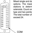
Mixed single and double wiring are available as options. The maximum number of manifold stations is determined by the number of solenoids. Count one point for a single solenoid type and two points for a double solenoid type. The total number of solenoids (points) must not exceed 24
