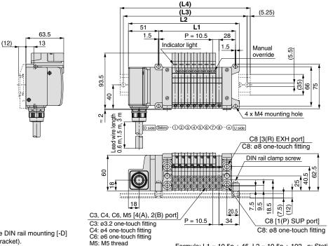
The dashed lines indicate DIN rail mounting [-D] (with DIN rail mounting bracket).
