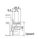
DIN rail mounting bracket [-D] VVQ1000-57A {For F/L/M/P/S (EX500) kit} VVQC1000-57A-S {For S (EX250) kit} VVQC1000-57A-T (For T kit)
