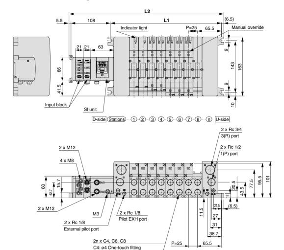
Formulas: L1 = 25n + 106, L2 = 25n + 205 (For one input block. Add 21 mm for each additional input block.) n: Stations (Maximum 16 stations)
