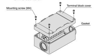
Step 3. How to replace the terminal block cover
