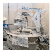
In addition to the requirements from UL and the FDA, cables in food and beverage applications must be able to withstand repeated washdown with a wide variety of chemicals. If a cable cannot withstand frequent washdown cycles, the cable jacket may become degraded. A damaged cable jacket will ultimately lead to cable failure and may pose a safety hazard. For this reason, cables for the food and beverage industry should be certified for washdown resistance.
